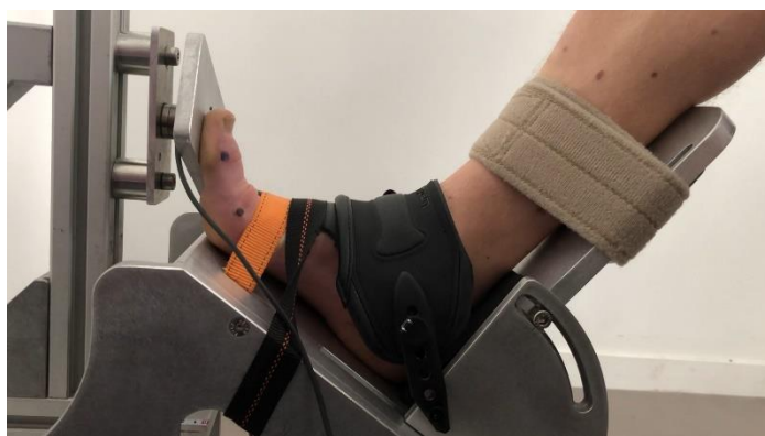
Figure 2 : Laboratory custom-built dynamometer evaluating MTP plantarflexion strength with a 3D forces sensor.
